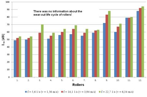
Fig. 6. Noise output levels measurements combined
