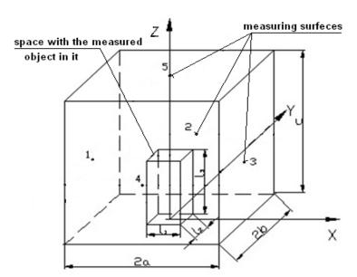
Fig. 2. Test arrangement for measurements conducted in an enclosed space
