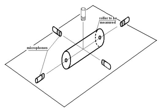
Fig. 3. Arrangement of the pick-ups during measurements
