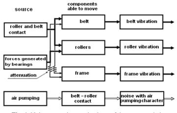
Fig. 1. Noise generating mechanisms of the conveyor belts
